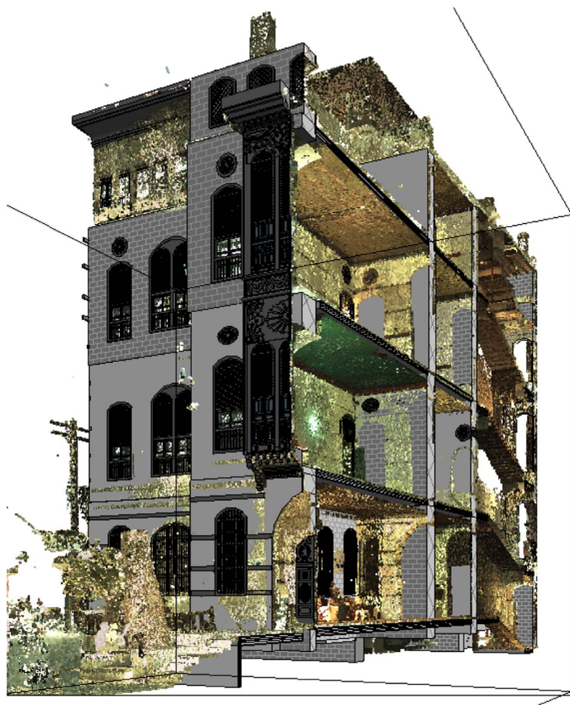
Fig. 21. 3D section on the JHBIM model and the point cloud.
