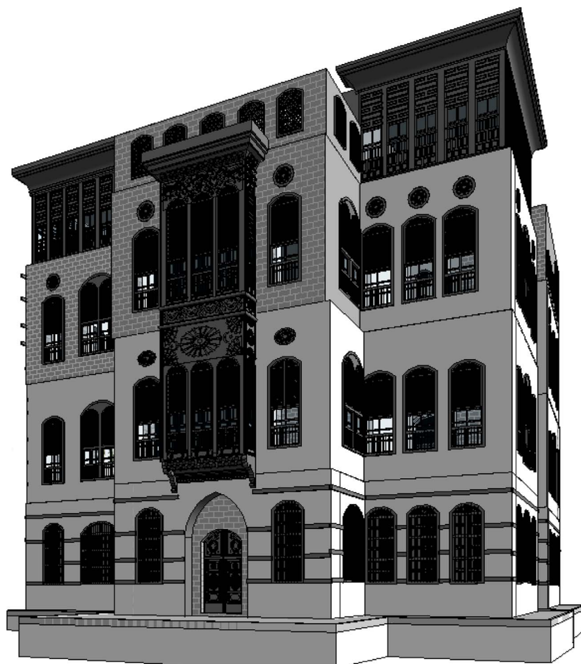
Fig. 20. 3D model of Nasif Historical House based on JHBIM.
