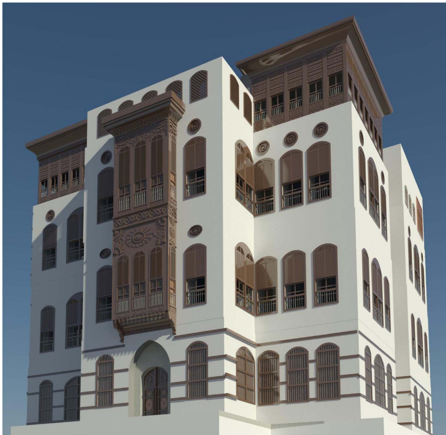
Fig. 22. Nasif Historical House JHBIM model after the rendering in Autodesk Revit.
