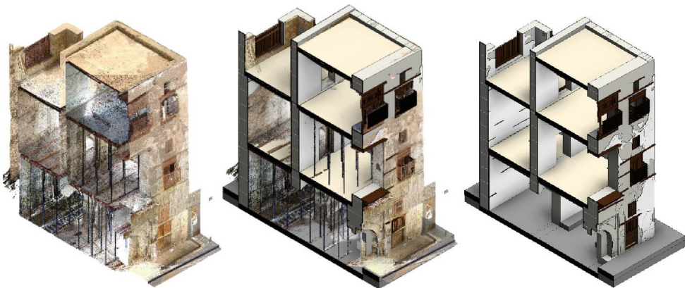
Fig. 10. The vertical section shows the HBIM modelling process
