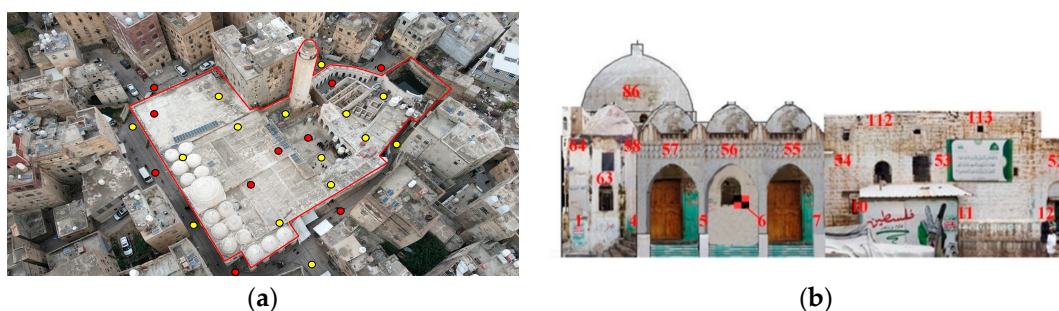
Figure 13. Distribution of GCPs (a) across the mosque during the UAVDP survey; (b) around the mosque during the TDP survey.
