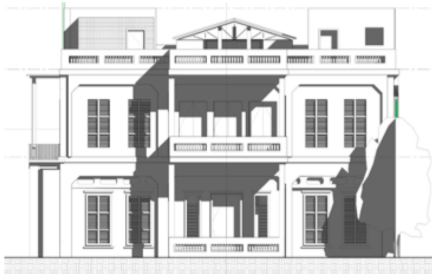
Figure 9. HBIM model developed directly from the point cloud data, illustrating the transition from scan-based documentation to information-rich modelling.
