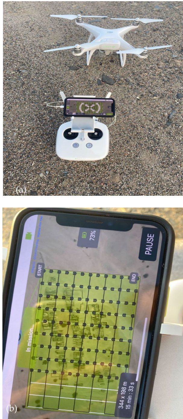
Figure 12. The process of aerial surveying: (a) DJI Phantom 4, and (b) Pix4D capture.
