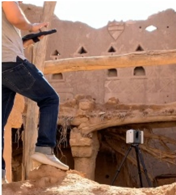
Fig. 13 High-fidelity 3D laser scanning of traditional Najdi architectural components, capturing geometric and material fidelity for HBIM integration
