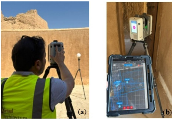
Fig. 14 Onsite 3D laser scanning workflow: (a) initial scan setup with spherical targets for registration, (b) pre-registration using Cyclone Field 360 software
