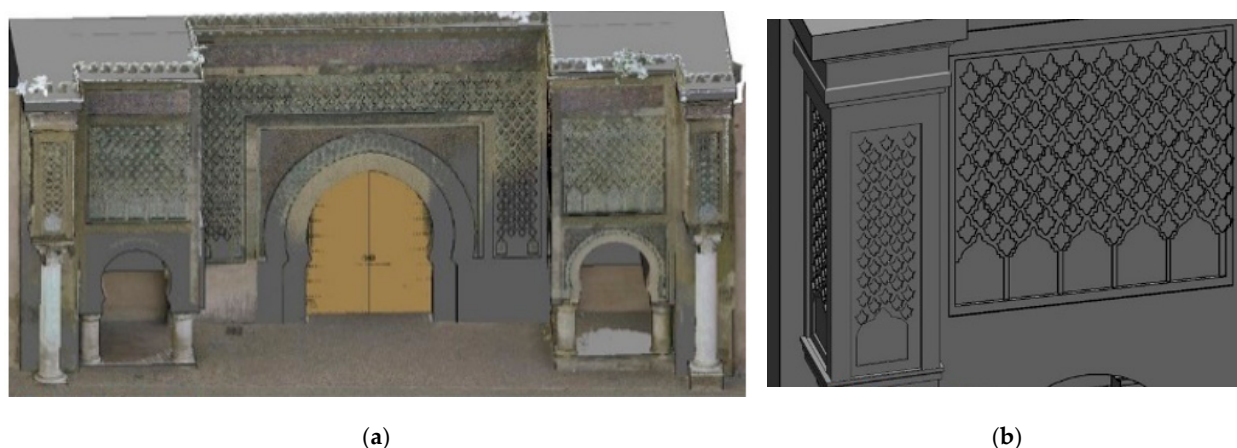
Figure 13. (a) Structural representation of Al-Mansour Gate for Digital Twin modeling and (b) textural information modeling from cloud point of Bab Al-Mansour.
