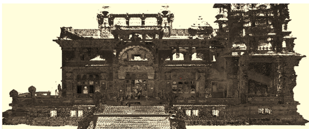
Figure 20. Filtration and registration of 23 scans of 12,702,112 points as a real image in RiSCAN.
