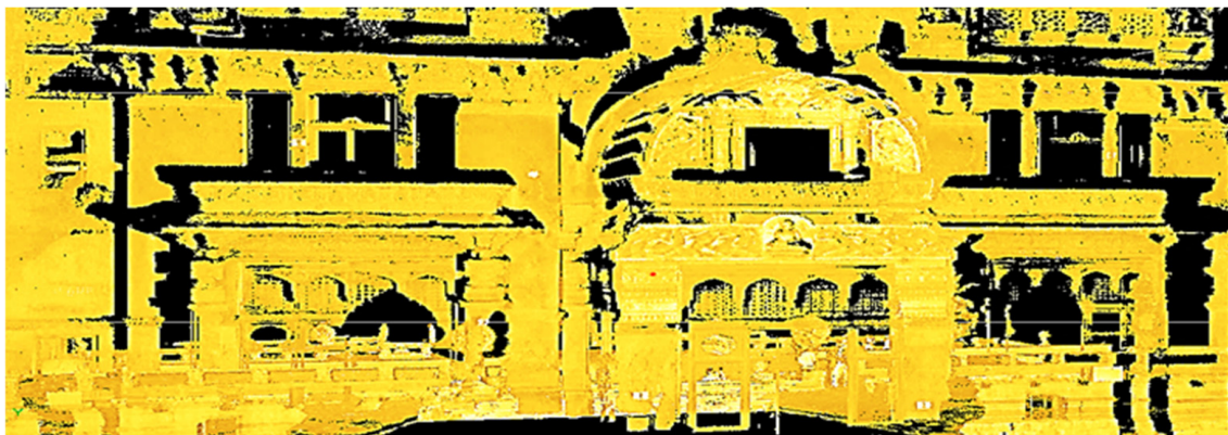
Figure 24. (16,297,294) points of 3D laser scan of Baron Palace façade in RiSCAN software.
